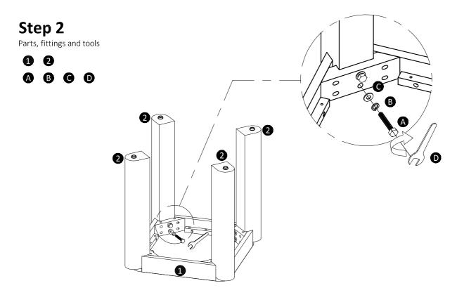
Insert x 1 bolt (A) x 1 spring washer (B) x 1 washer (C) combine together as shown above and tighten with the wrench (D) provided. Repeat with each of the four legs (x4)
