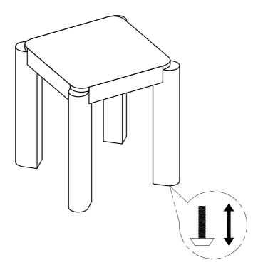
Turn the adjustable feet to allow the table to stand flat on the floor
