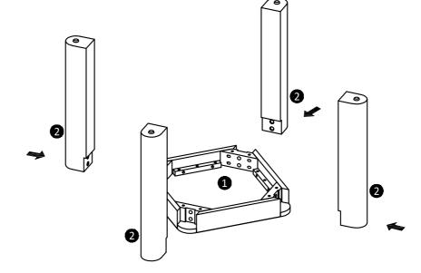
Find a clear area for assembly, near where you intend to use the table. Place the table top (1) upside down on a soft surface, being careful not to damage the finish. Taking legs (2), turn upside down and locate into the table top (1) as shown.
