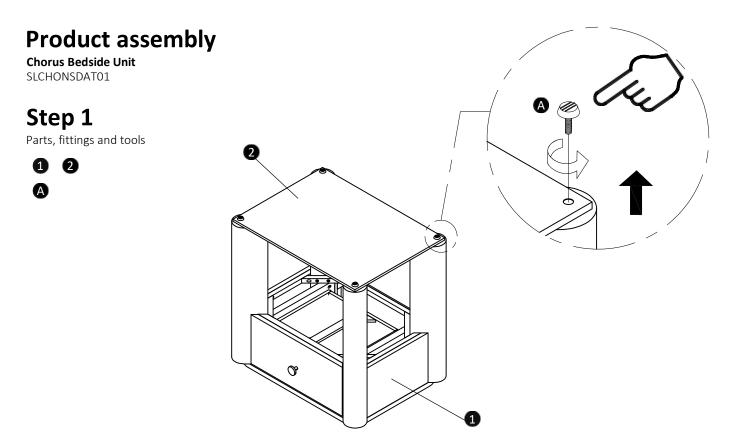
Find a clear area for assembly, near where you intend to use the table. Place the table upside down on a soft surface, being careful not to damage the finish. Remove the adjustable feet, and then detach the bottom panel from the table.
