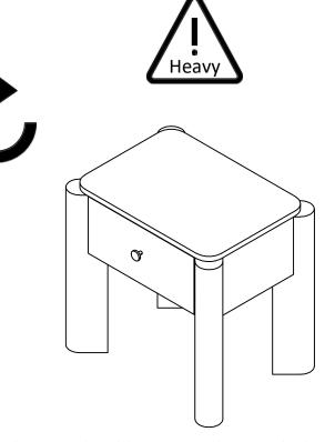
With 1 person carefully place the table on its feet. Take care when lifting not to damage the legs.
