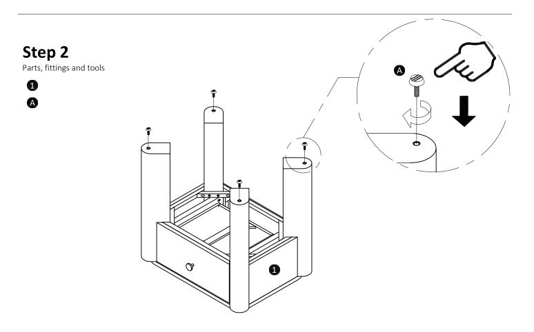
Insert **Adjustable feet A** as shown above. Repeat with each of the four legs (x4)
