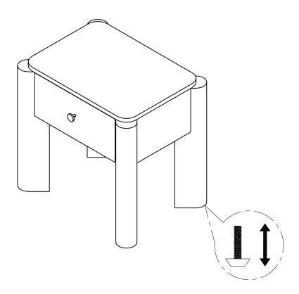
Turn the adjustable feet to allow the table to stand flat on the floor
