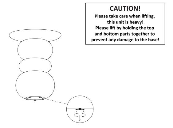
Carefully lift the table and turn the adjustable feet on the base to level the product.
