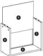
Attach left drawer (7) and right dawer (8) to rear drawer (6) using screws (G). Insert bottom drawer (9) into assembly drawer as shown.
