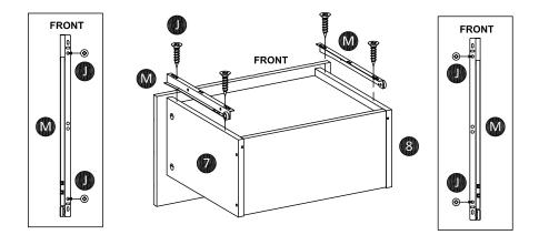
Attach drawer rail (M) to left drawer (7) and right drawer (8) using screw (J).
