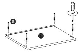
Attach cam-bolt (B) to top panel (1) using screwdriver.
