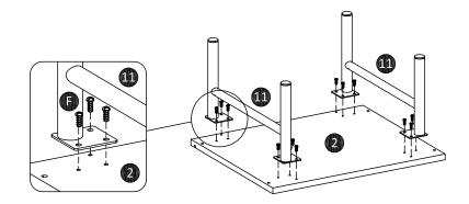
Attach metal leg (11) to bottom panel (2) using screw (F) as shown.
