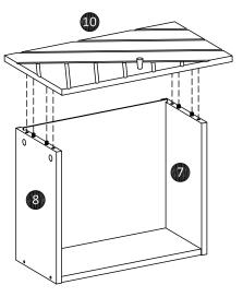
Attach front drawer (10) to assembly drawer as shown. Turn the cam-lock (A) clockwise to lock using screwdriver, then paste cam-sticker (D).
