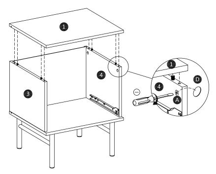
Attach top panel (1) to case assembly as shown. Turn the cam-lock (A) clockwise to lock using screwdriver, then paste cam-sticker (D).
