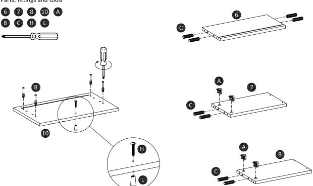
Attach cam-bolt (B) to front drawer (10) using screwdriver and attach handle (L) to front drawer (10) using screw (H) as shown. Insert cam-lock (A) into left drawer (7) and right drawer (8). Insert plastic dowel (D) into rear drawer (6), left drawer (7) and right drawer (8).
