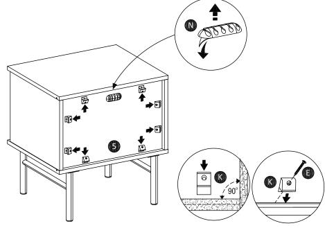
Attach backply stopper (K) to backboard (5) using screw (E). Paste cable clamp (N) on the backboard (5) as shown.
