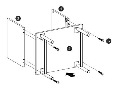
Attach left panel (3) and right panel (4) to bottom panel (2) using screw (G) as shown.
