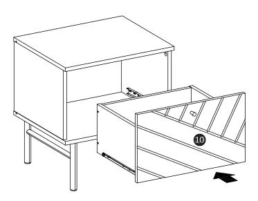
Insert assembly drawer into case assembly as shown.
