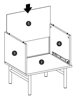
Insert backboard (5) into case assembly as shown.
