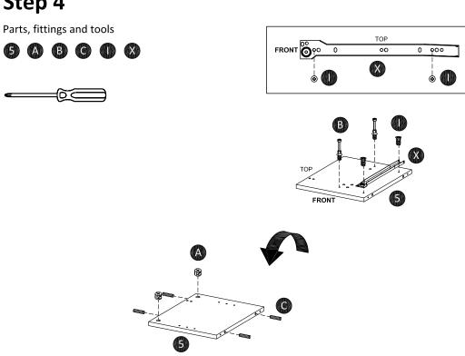
Attach cam-bolt (B) to left divider (5) using screwdriver, then insert cam-fix (A) and plastic dowel (C). Attach drawer rail (X) to left divider (5) using screw (I).
