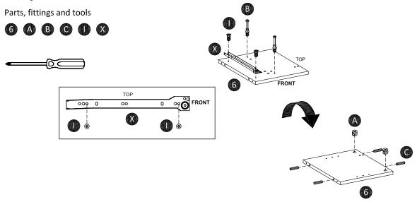
Attach cam-bolt (B) to right divider (6) using screwdriver, then insert cam-fix (A) and plastic dowel (C). Attach drawer rail (X) to right divider (6) using screw (I).
