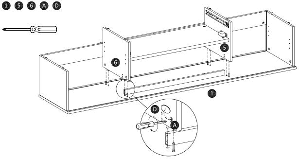
Attach divider assembly to case assembly as shown. Turn the cam-lock (A) clockwise to lock using screwdriver, then paste cam-sticker (D).
