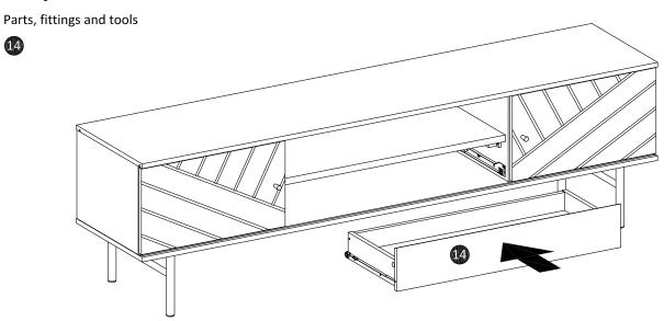
Insert assembly drawer into case assembly as shown.
