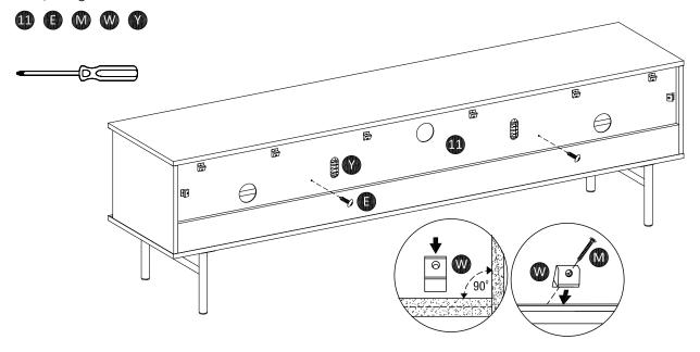
Attach backply stopper (W) to backboard (11) using screw (M). Strenghten backboard (11) with screw (E) as shown. Paste cable clamp (Y) on the backboard (11) as shown.
