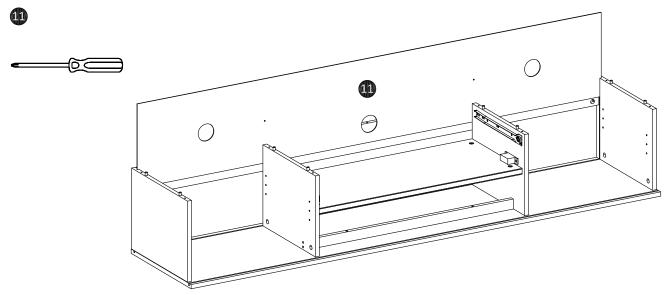
Insert backboard (11) into case assembly as shown.
