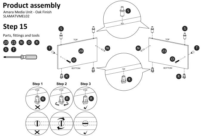
Insert push pin (S) in top of left door (20) and right door (21) while fix pin (R) in the bottom as shown. Insert door stopper (N) in the left door (20) and right door (21) as shown. Attach handle (T) to left door (20) and right door (21) using screw (O).
