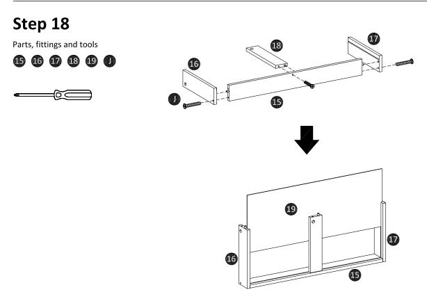
Attach left drawer (16) and right dawer (17) to rear drawer (15) using screws (J). Insert bottom drawer (19) into assembly drawer as shown.
