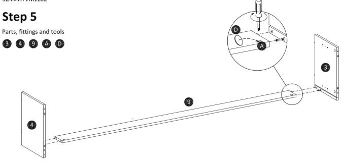
Attach left panel (3) and right panel (4) to rear panel (9) as shown. Turn the cam-lock (A) clockwise to lock using screwdriver, then paste cam-sticker (D).
