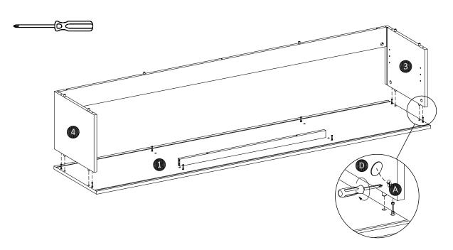
Attach case assembly to top panel (1) as shown. Turn the cam-lock (A) clockwise to lock using screwdriver, then paste cam-sticker (D).
