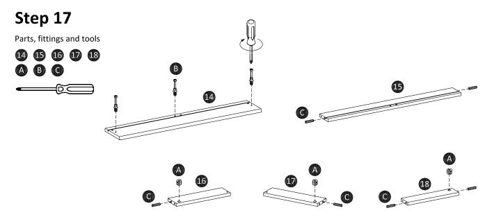
Attach cam-bolt (B) front drawer (14) using screwdriver. Insert cam-lock (A) into left drawer (16), right drawer (17) and bottom support drawer (18). Insert plastic dowel (C) into rear drawer (15), left drawer (16) and right drawer (17).
