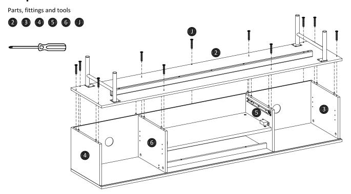
Attach bottom panel (2) to case assembly using screw (J).
