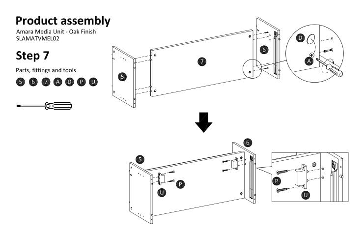
Attach left divider (5) and right divider (6) to fix shelf (7) as shown. Turn the cam-lock (A) clockwise to lock using screwdriver, then paste cam-sticker (D). Attach Drawer stopper (U) to left divider (5) and right divider (6) using screw (P).
