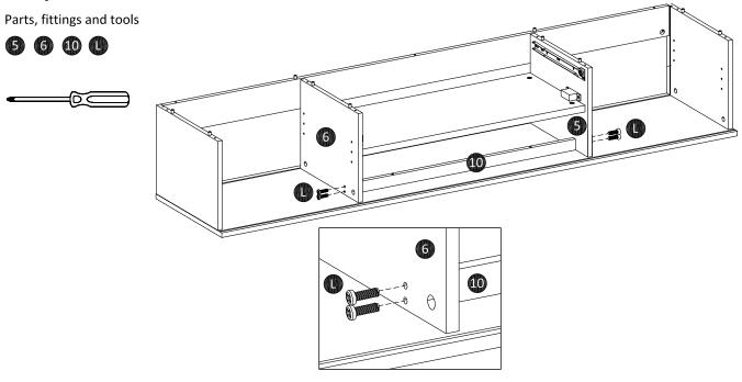
Strenghten top metal support (10) with the divider using screw (L).
