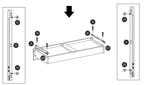
Attach front drawer (14) to assembly drawer as shown. Turn the cam-lock (A) clockwise to lock using screwdriver, then paste cam-sticker (D). Attach drawer rail (X) to left drawer (16) and right drawer (17) using screw (H).
