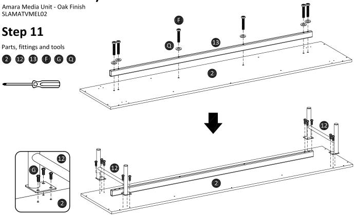
Attach bottom metal support (13) to bottom panel (2) using screw (F) and washer (Q). Attach metal leg (12) to bottom panel (2) using screw (G).
