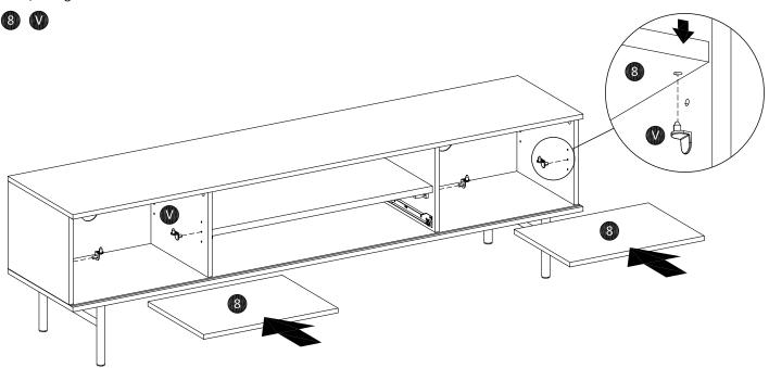
Insert shelf support (V) into case assembly as shown. Insert adjustable shelf (8) into case assembly as shown.
