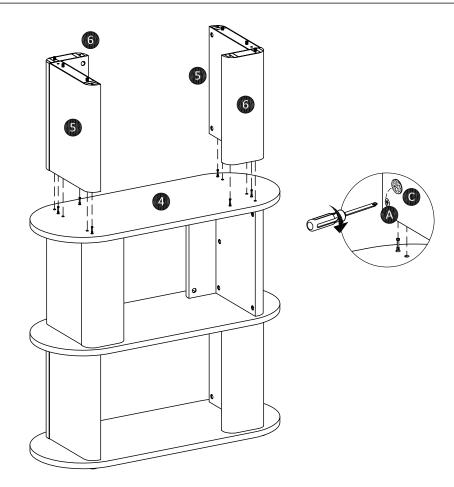
Attach side panel and divider to middle panel (4) as shown. Turn the cam-lock (A) clockwise to lock using screwdriver, then paste cam-sticker (C).
