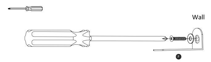
Secure the wall brackets (F) to the wall using the washers (not included) and screws (not included). Tighten with the screwdriver.
