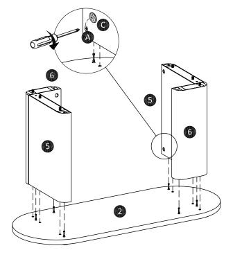
Attach side panel and divider to bottom panel (2) as shown. Turn the cam-lock (A) clockwise to lock using screwdriver, then paste cam-sticker (C).
