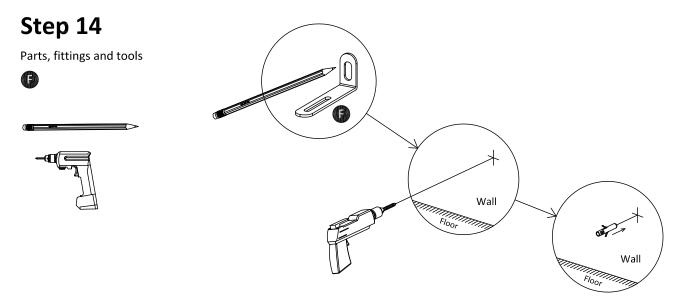
Reposition the wall bracket with a pencil where the screw holes are going to be located. Before drilling, ensure the size of holes will be correct to fit the rawl plugs (not included).
