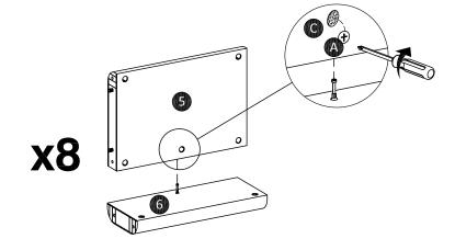
Attach side panel (5) to side support (6) as shown. Turn the cam-lock (A) clockwise to lock using screwdriver, then paste cam-sticker (C).
