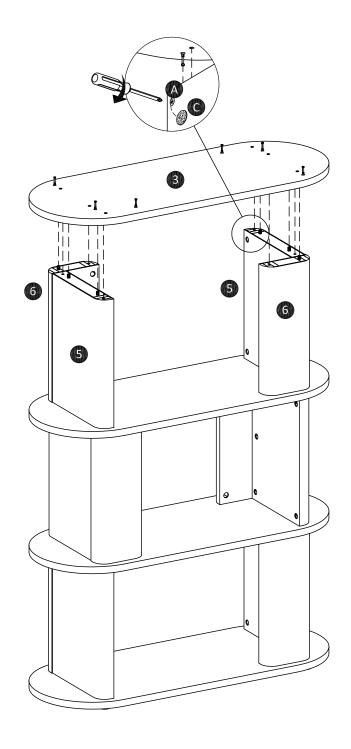
Attach top/bottom middle panel (3) to case assembly as shown. Turn the cam-lock (A) clockwise to lock using screwdriver, then paste cam-sticker (C).
