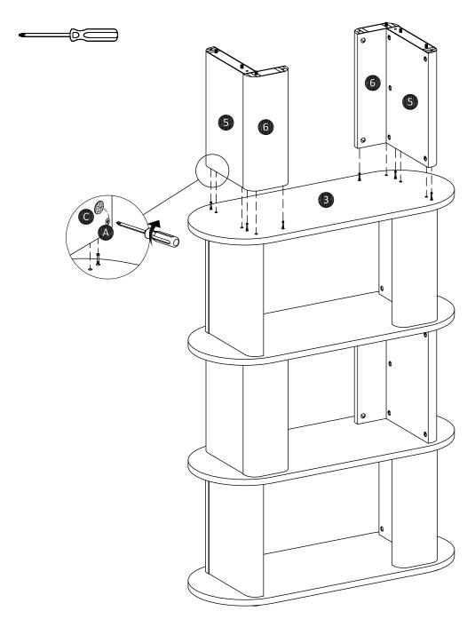
Attach side panel and divider to top/bottom middle panel (3) as shown. Turn the cam-lock (A) clockwise to lock using screwdriver, then paste cam-sticker (C).
