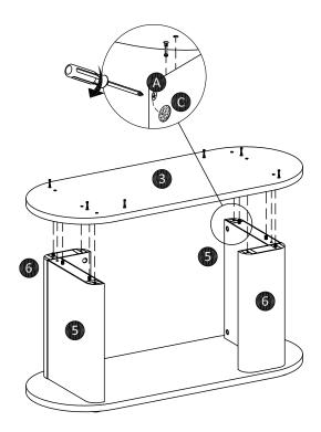
Attach top/bottom middle panel (3) to case assembly as shown. Turn the cam-lock (A) clockwise to lock using screwdriver, then paste cam-sticker (C).
