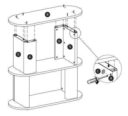
Attach middle panel (4) to case assembly as shown. Turn the cam-lock (A) clockwise to lock using screwdriver, then paste cam-sticker (C).
