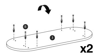
Attach cam-bolt (B) to top/bottom middle panel (3) using screwdriver. Flip the panel  $180^\circ$  and then attach again cam-bolt (B) as shown.
