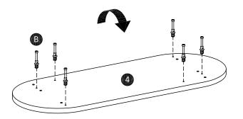
Attach cam-bolt (B) to middle panel (4) using screwdriver. Flip the panel 180° and then attach again cam-bolt (B) as shown.
