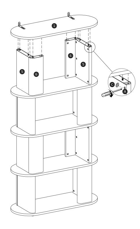
Attach top panel (1) to case assembly as shown. Turn the cam-lock (A) clockwise to lock using screwdriver, then paste cam-sticker (C).
