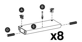
Attach cam-bolt (B) to bottom panel (2) and side support (6) using screwdriver. Insert cam-fix (A) and plastic dowel (D) into side panel (5) and side support (6).
