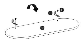
Attach cam-bolt (B) to top panel (1) using screwdriver. Flip top panel 180° then attach wall brackets (F) using screws (E).
