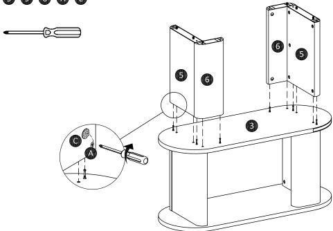
Attach side panel to top/bottom middle panel (3) as shown. Turn the cam-lock (A) clockwise to lock using screwdriver, then paste cam-sticker (C).
