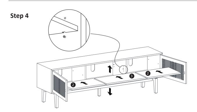
Locate the shelves (2), (3) at the desired height onto the shelf pins as shown above.
