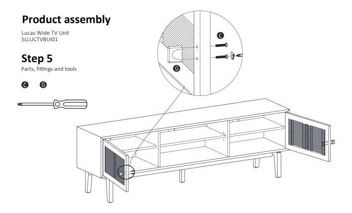
Locate the handles (G) as shown above and secure with the crosshead screws (C) using the screwdriver. Take care when installing to not scratch the handle finish. Hinges have been preadjusted, do not adjust. Repeat with the two doors (x2).
