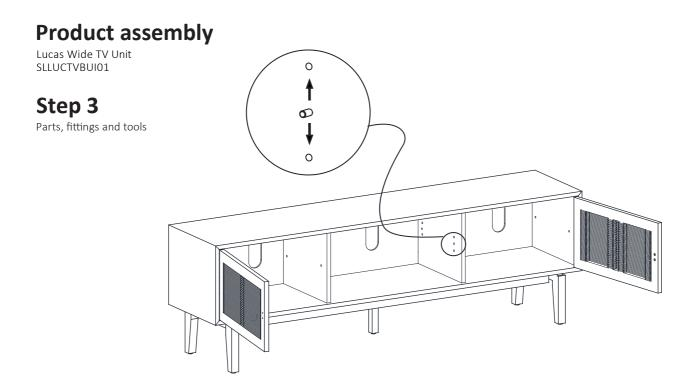
Open the doors, choose the height you'd like the central shelf to be at, and adjust the shelf height by unscrewing and repositioning the shelf pins up and/or down in the given holes.
