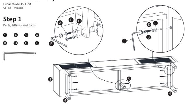
carefully lie the cabinet on its back onto the soft surface. Attach the side legs (4) and the central leg (5) as shown in the image above using the bolt (B) for the side legs, bolt (A) for the central leg, flat washer (D), lock washer (E) and tighten with Allen key (F).
