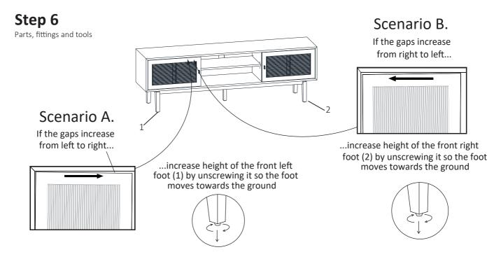
Move the cabinet into its location of intended use next to a wall. Turn the adjustable feet so the cabinet is level (you can use a spirit level to help here). Also check that the doors are level - the gap between the top edge of the doors and the frame above should ideally be consistent. If it is not, you can correct this by making slight adjustments to the feet by following the guide above.
