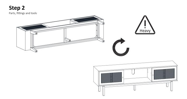
With 2 people carefully place the cabinet on its feet. Take care when lifting not to damage the legs.
