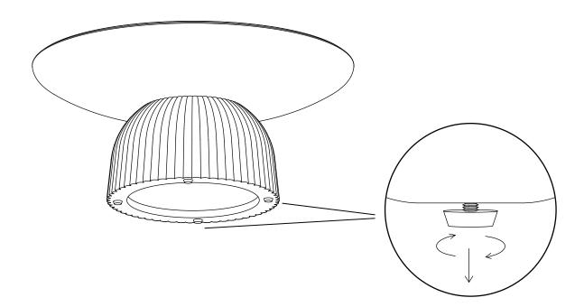
Carefully lift the table and turn the adjustable feet on the base to level the product.
