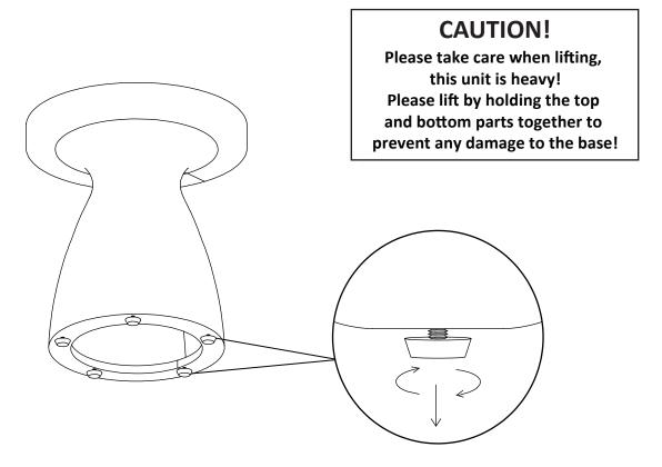
Carefully lift the table and turn the adjustable feet on the base to level the product.
