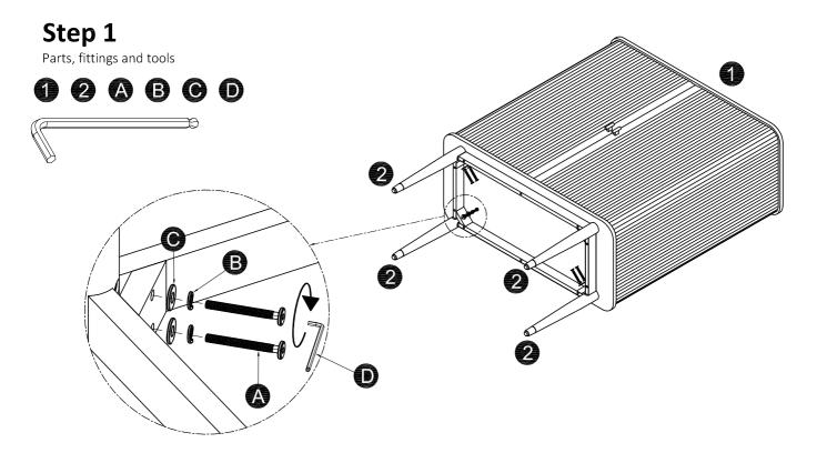
Find clear area for assembly, near where you intend to use the bar cabinet. Turn the table top upside down. Use x1 small allen bolt (A) x 1 lock washer (B) and x 1 washer (C) combine together as shown above and tighten with allen key (D) provided. Repeat with each of the four legs (x4).
