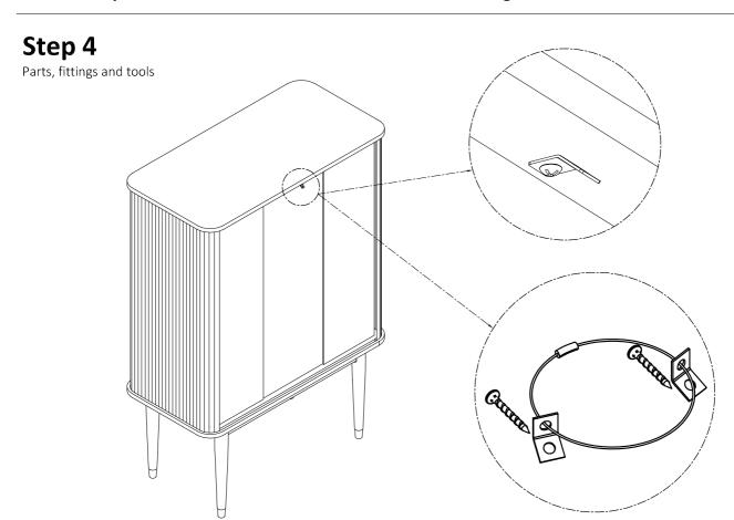
REMARK: There is a tip restraint kit provided on the back of this product please read the direction thoroughly and install immediately. Attach the Anti-tip Kit to the top cabinet (in back).
