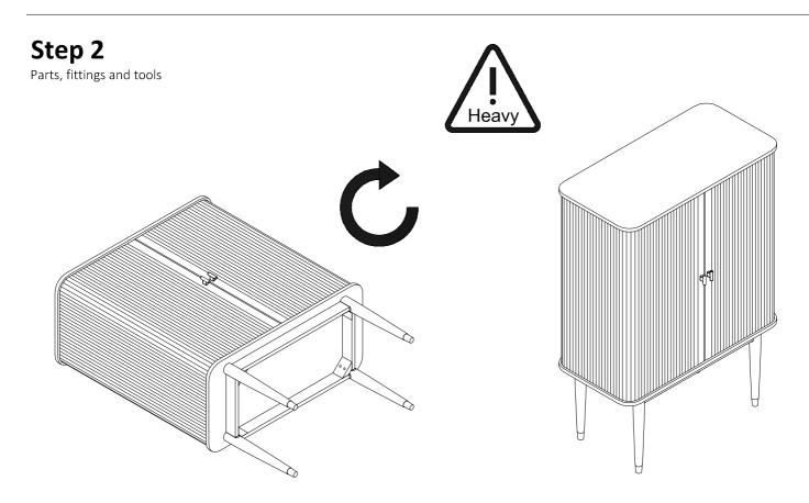
With 2 people carefully place the table on its feet. Take care when lifting not to damage the legs.
