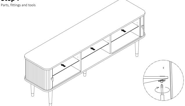
Carefully slide the glass shelf into the cabinet resting on the plastic grub screws of each shelf clip. Then tighten plastic grub screws from below to secure shelf in place.
