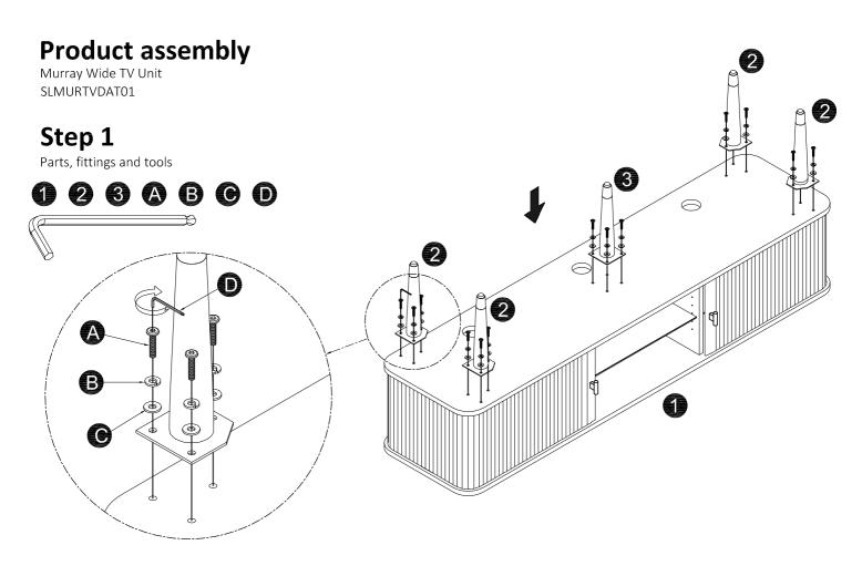
Find clear area for assembly, near where you intend to use the TV Unit. Turn the top cabinet upside down on a soft surface. Then insert x1 small allen bolt (A) x1 lock washer (B) and x1 washer (C) combine together as shown above and tighten with allen key (D) provided. Repeat with each of the five legs (x5).
