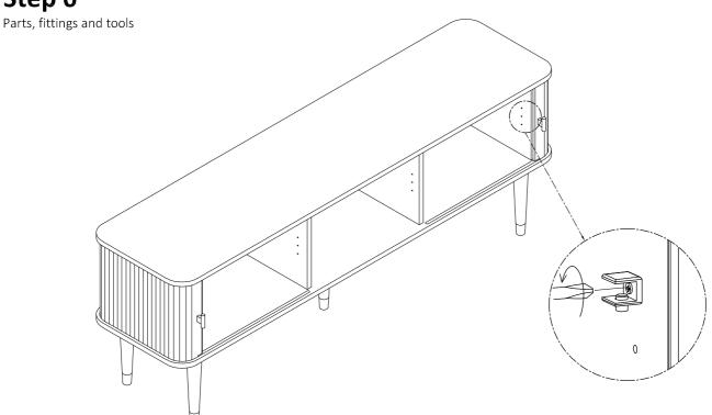
Put in shelf clips for each shelf at desired height ensuring the plastic grub screw is towards the base. Give the screw a half turn clockwise to tighten in place
