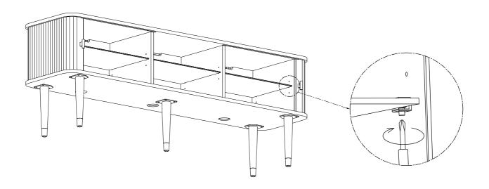
Adjustable shelf to the desired height by unscrewing the plastic grub screws from below
