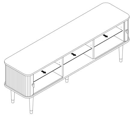
Carefully slide the glass shelf out of the plastic grub screws of each shelf clip
