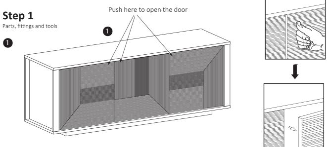
Open the door and take out the legs and the shelves inside. The fittings bag is located inside the box with legs.
