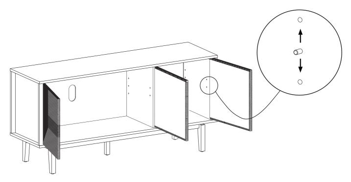
Open the doors, choose the height you'd like the shelves to be at, and adjust the shelf height by unscrewing and repositioning the shelf pins up and/or down in the given holes.
