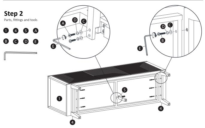
carefully lie the cabinet on its back onto the soft surface. Attach the legs as shown in the image above using bolts (B) for the side legs, bolts (A) for the central leg, flat washer (C), lock washer (D), and tighten with Allen key (E).
