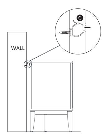
Reposition the cabinet back in place so that the cable tie mounts are aligned. Feed the Cable ties (G) through both Cable tie mounts. Then push the cabinet against the wall and pull the cable ties.
