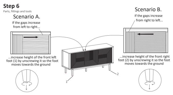
Move the cabinet into its location of intended use next to a wall. Turn the adjustable feet so the cabinet is level (you can use a spirit level to help here). Also check that the doors are level - the gap between the top edge of the doors and the frame above should ideally be consistent. If it is not, you can correct this by making slight adjustments to the feet by following the guide above.
