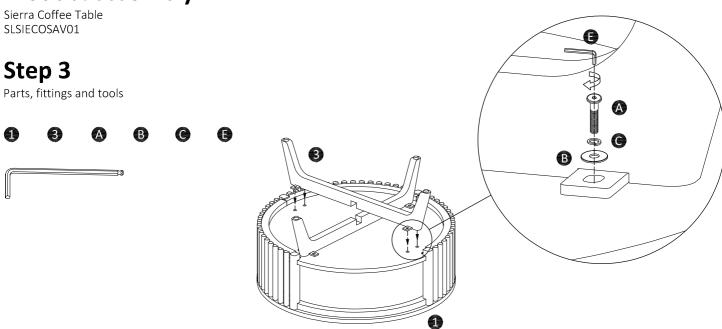
Use the allen bolt (x4 part A), washers (x4 part B) and lock washers (x4 part C) to fix the lower leg (3) onto the cabinet as shown above. Tighten with the allen key (E)
