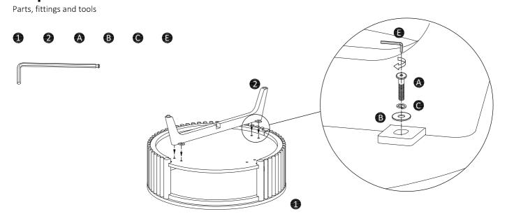
Find a clear area for assembly, near where you intend to use the coffee table. Place the cabinet (1) upside down on a soft surface. Then use the allen bolt (x4 part A), washers (x4 part B) and lock washers (x4 part C) to fix the upper leg (2) onto the cabinet as shown above. Tighten with the allen key (E).
