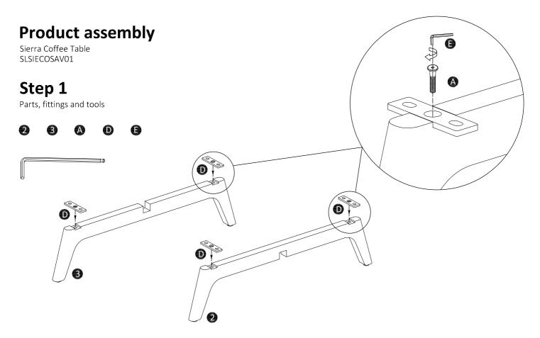
Use the allen bolts (x2 part A) and the allen key (E) to fix the barcket (x2 part D) to the upper leg (2). Do the same for the lower leg (3)
