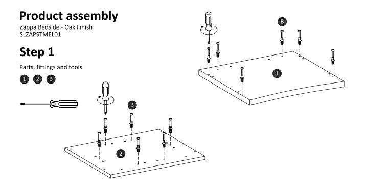
Attach cam-bolt (B) to top panel (1) and bottom panel (2) using screwdriver.
