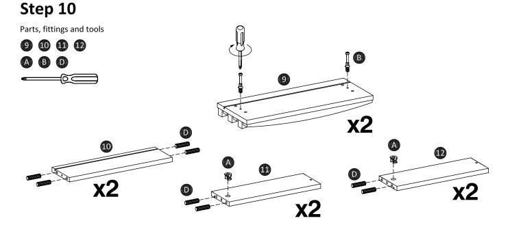
Attach cam-bolt (B) to front drawer (9) using screwdriver. Insert cam-lock (A) into left drawer (11) and right drawer (12). Insert plastic dowel (D) into rear drawer (10), left drawer (11) and right drawer (12).
