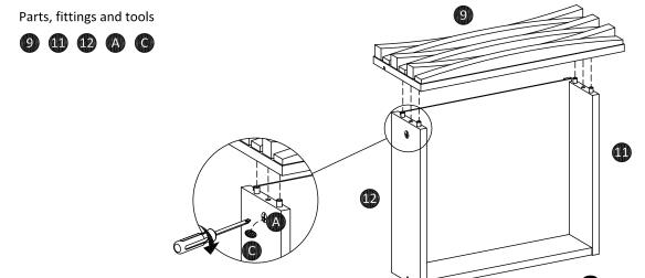
Attach front drawer (9) to assembly drawer as shown. Turn the cam-lock (A) clockwise to lock using screwdriver, then paste cam-sticker (C).
