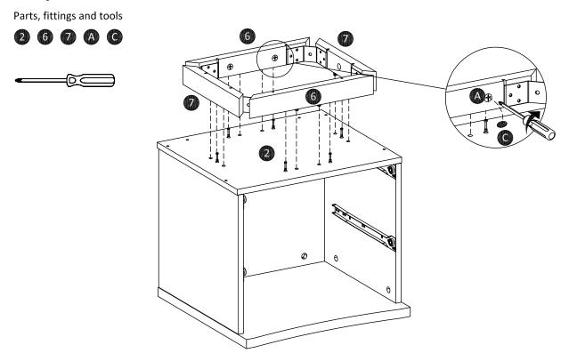
Attach support assembly to bottom panel (2) as shown. Turn the cam-lock (A) clockwise to lock using screwdriver, then paste cam-sticker (C).
