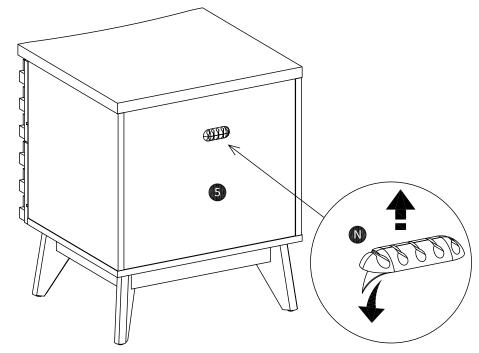
Paste cable clamp (N) on the rear panel (5) as shown.
