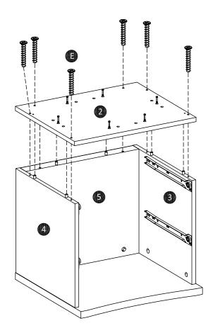
Attach bottom panel (2) to case assembly using screws (E) as shown.
