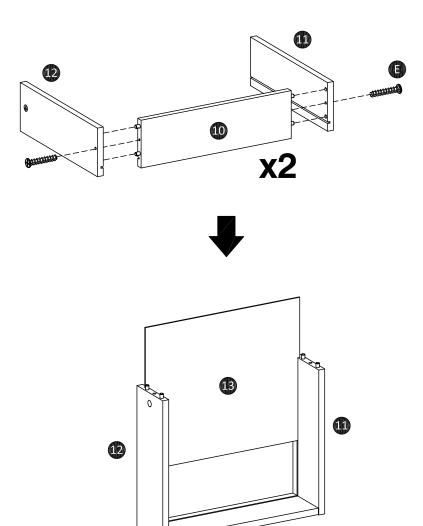
Attach left drawer (11) and right dawer (12) to rear drawer (10) using screws (E). Insert bottom drawer (13) into assembly drawer as shown.
