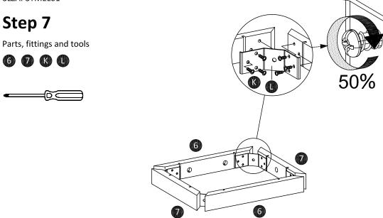
Attach corner brace (L) on the between large support (6) and small support (7) using screws (K). Tighten the screws about 50% before fixed.
