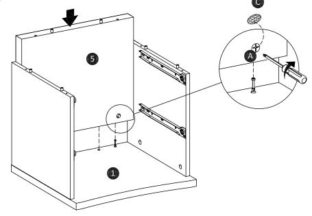
Attach rear panel (5) to case assembly as shown.
