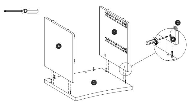
Attach left panel (3) and right panel (4) to top panel (1) as shown. Turn the cam-lock (A) clockwise to lock using screwdriver, then paste cam-sticker (C).
