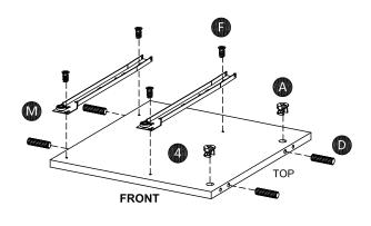
Insert cam-fix (A) and plastic dowel (D) into left panel (3) and right panel (4). Attach drawer rails (M) to left panel (3) and right panel (4) using screws (F).
