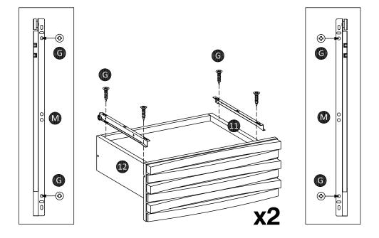
Attach drawer rail (M) to left drawer (11) and right drawer (12) using screw (G).
