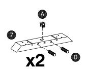
Insert cam-fix (A) and plastic dowel (D) into rear panel (5), large support (6) and small support (7).
