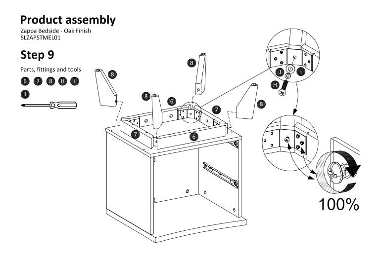
Attach leg (8) in the between large support (6) and small support (7), then screws the legs from corner brace using screws (H), washer plate (I) and washer (J) as shown. Tighten screws (K) around corner brace and fixed it.
