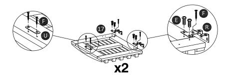
Attach door hinge (M) on the side door (16) using screws (E). Attach plate hinge (R) on the Middle door (17) using screws (E) and (F), then install plate (U) using screws (F).
