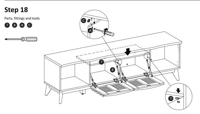
Insert fix shelf (7) into case assembly as shown. Turn the cam-lock (A) clockwise to lock using screwdriver, then paste cam-sticker (C).
