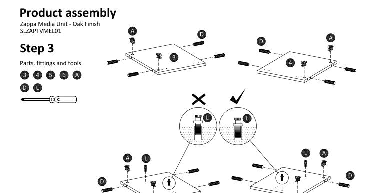
Insert cam-fix (A) and plastic dowel (D) into left panel (3), right panel (4), left divider (5) and right divider (6). Attach shelf holder (L) to left divider (5) and right divider (6) as shown.
