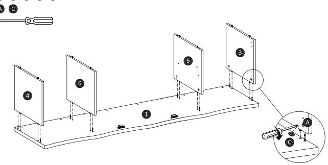
Attach left panel (3), right panel (4), left divider (5) and right divider (6) to top panel (1). Turn the cam-lock (A) clockwise to lock using screwdriver, then paste cam-sticker (C).
