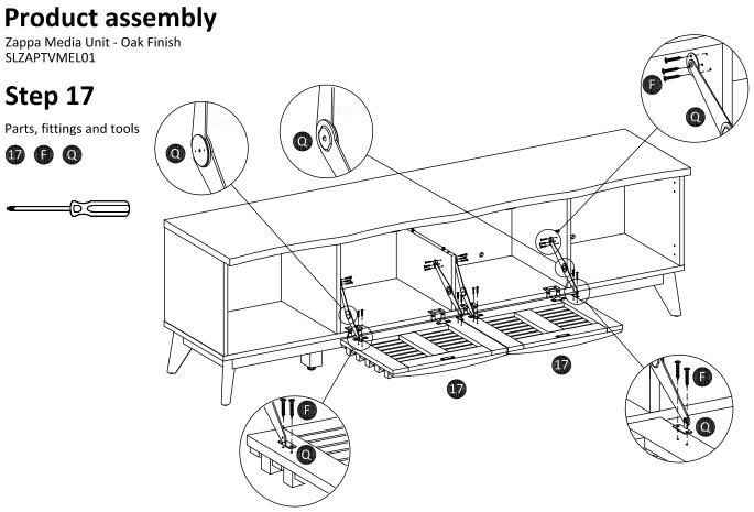
Attach flap stay (Q) on the middle door (17) then screw it using screws (F) as shown.
