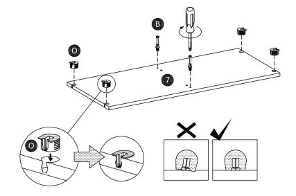
Attach cam-bolt (B) to fix shelf (7) using screwdriver. Insert shelf support (O) into fix shelf (7) as shown.
