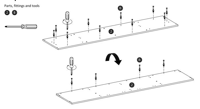
Attach cam-bolt (B) to bottom panel (2) using screwdriver. Flip the panel 180°, then attach again cam-bolt (B) using screwdriver as shown.
