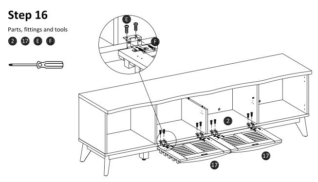
Attach middle door (17) to bottom panel (2), then screw the plate hinge (R) using screws (E) and (F) as shown.
