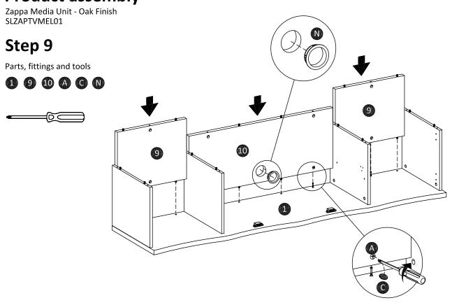
Attach side rear panel (9) and middle rear panel (10) to case assembly as shown. Turn the cam-lock (A) clockwise to lock using screwdriver, then paste cam-sticker (C). Insert cable holder (N) into middle rear panel (10).
