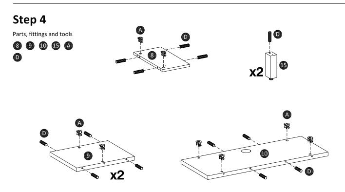
Insert cam-fix (A) and plastic dowel (D) into middle divider (8), side rear panel (9) and middle rear panel (10). Insert plastic dowel (D) into middle leg (15).
