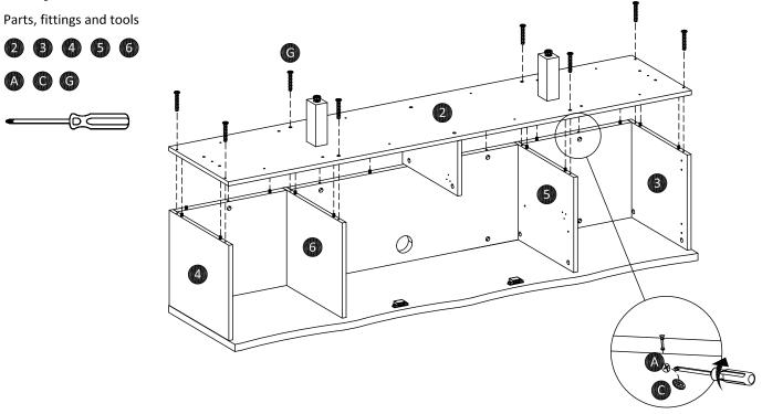
Attach bottom panel (2) to case assembly using screws (G). Turn the cam-lock (A) clockwise to lock using screwdriver, then paste cam-sticker (C).
