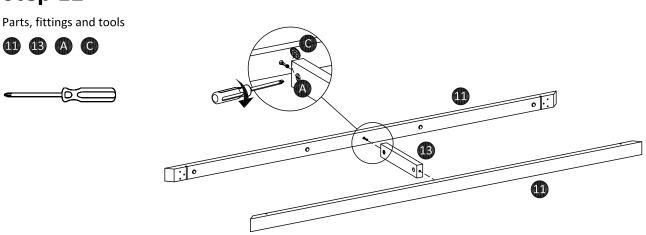
Attach large support (11) to middle support (13) as shown. Turn the cam-lock (A) clockwise to lock using screwdriver, then paste cam-sticker (C).
