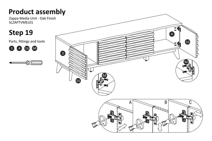
Attach side door (16) to case assembly, then thightening the screws using screwdriver. Adjust the hinge on the door until fix with the assembly.
