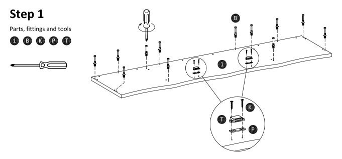
Attach cam-bolt (B) to top panel (1) using screwdriver. Attach magnet (T) and magnet support (P) using screws (K).
