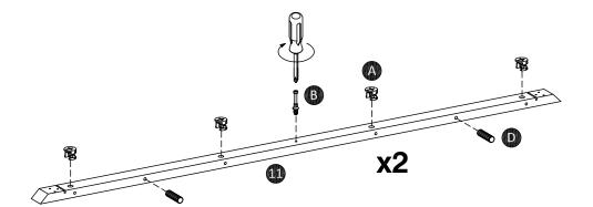
Attach cam-bolt (B) to large support (11) using screwdriver. Insert cam-fix (A) and plastic dowel (D) into large support (11), small support (12) and middle support (13).
