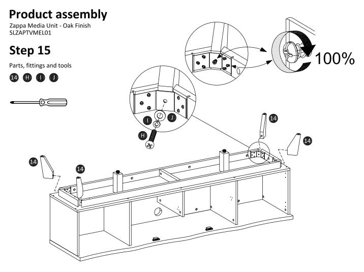
Attach side leg (14) on the between large support (11) and small support (12) using scews (H), washer plate (J) and washer (I). Tighten screws (E) around corner braces and fixed it.
