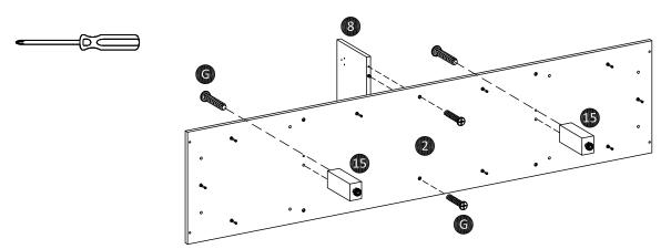
Attach middle legs (15) to bottom panel (2) using screws (G). Attach midde divider panel (8) to bottom panel (2) using screws (G).
